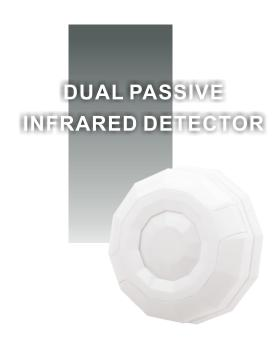
The Dual Passive Infrared Detector works through detecting the human body's infrared spectrum. While received the heat source signal from body's movement in the detecting area, the signal will be transmitted to the MCU after enlarged, MCU sends out the signal to control the alarm port after analyzed and calculated. The Detector is widely used in banks, warehouse, homes, etc.
